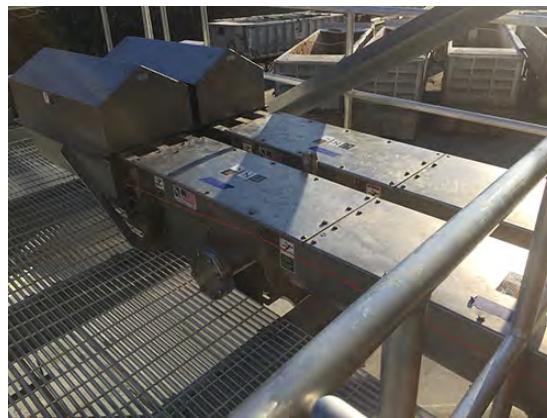
Drive Ends of KWS Shaftless Screw Conveyors are Protected from the Environment with Special Covers
