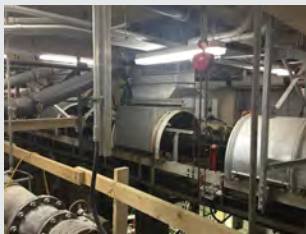
Existing Belt Conveyor was Removed and Replaced with KWS Shaftless Screw Conveyors
