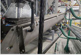
Thermal Processors Continuously Cool or Heat Bulk Materials
