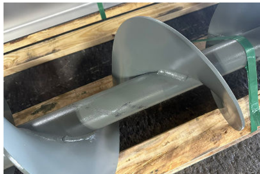
Screw Shown has Continuous Welding on Carrying Side and Skip Welds on Back Side of Flighting
