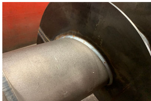
Continuous Welding on Carrying Side Connects Flighting to Center Pipe
