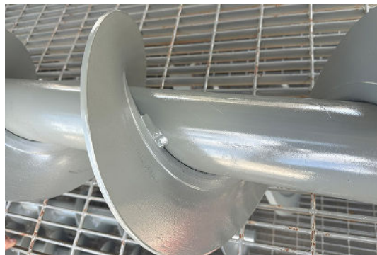
Typical Skip Welds are 2-Inch-Long Intermittent Welds on Every Other Flight
