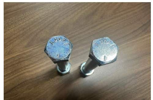
Grade 5 Coupling Bolts Deform Slightly and Absorb Energy Before Failure
