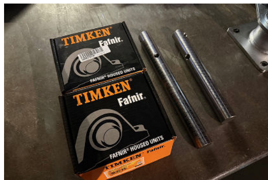
KWS Provided a Replacement Screw, Drive Shaft, End Shaft, and Two End Bearings
