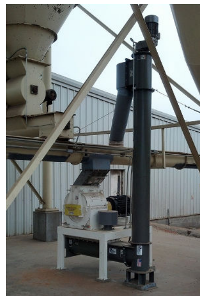
Understanding Bulk Material Characteristics and Other Factors are Important for Proper Vertical Screw Conveyor Design
