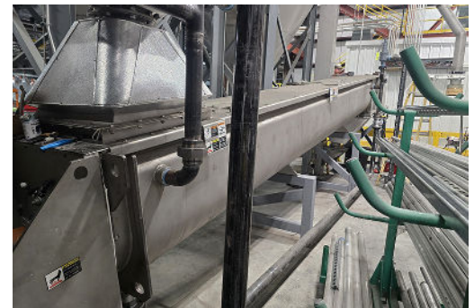
KWS Thermal Processors are Used to Cool or Heat Various Bulk Materials
