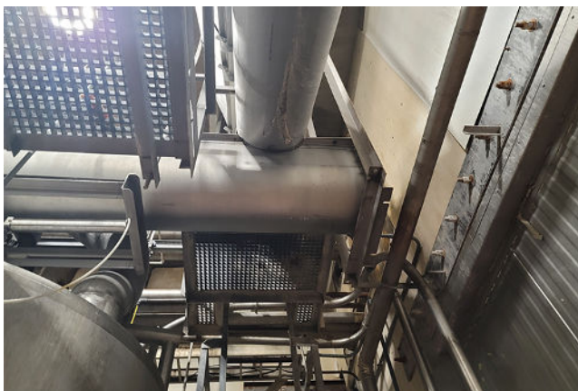
Limited Space Requires Two Screw Conveyors to be Coped
