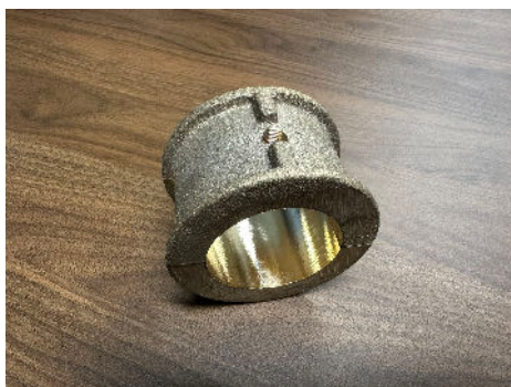
Bronze Hanger Bearings are Not Suitable for All Food-Grade Applications
