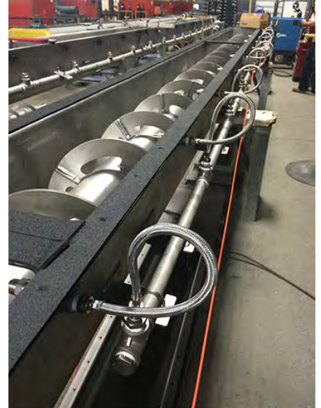
Figure 2: Spray Nozzles are Located in Side of Trough to Completely Clean Interior Surfaces
