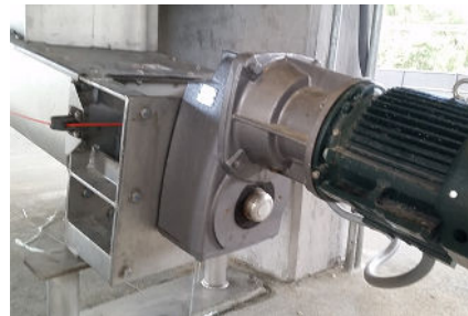
Screw Conveyor with Gear Reducer and Motor Can Be Anchored Directly to Foundation
