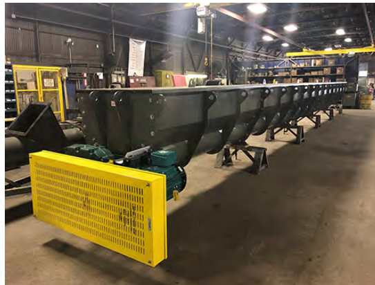
Offal Screw Feeders and Conveyors are Largest and Most Rugged in a Rendering Plant
