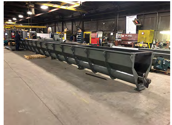
KWS Keyhole Trough Screw Conveyor Ready for Shipment
