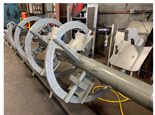
Post Type Ribbon Screw for Conveying Wet Chemicals and Salt
