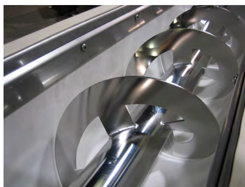
Stainless Steel Integral Post Ribbon Screw for Conveying Wet Starch
