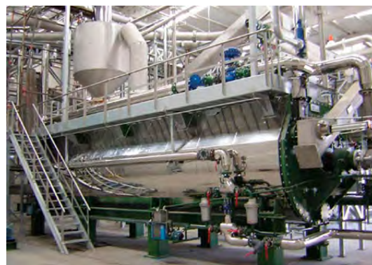
In the Rendering Process, Meat is Cooked to Separate Fats from Solids
