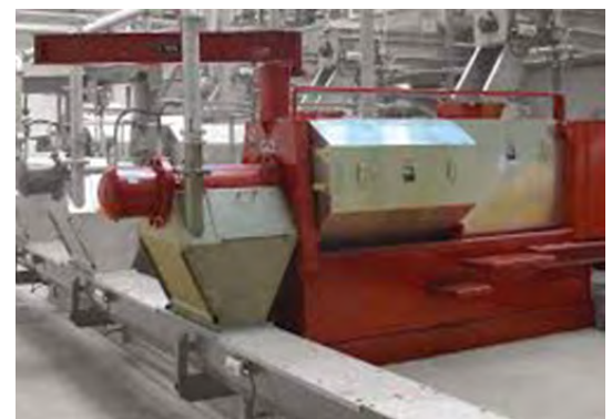
Multiple Screw Presses Remove Oil from Crax
