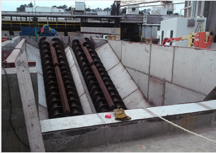
Large Meat Bin with Quad Screw Feeder and High Torque Drive Units
