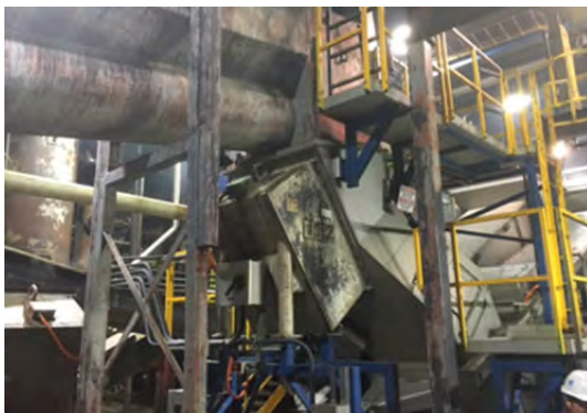
Keyhole Trough Conveys Raw Materials to Magnetic Separation and Grinding
