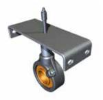
Style 670 hangers are an inside flush mounted hanger. Supplied with a dust-tight sealed ball bearing, style 670 hangers allow for 4-degrees of shaft misalignment and temperatures up to 240-degrees F. The pipe body bar provides rigidity for light and medium duty applications while allowing minimal obstruction of material flow. The flush mounted top bar bolts to the inside of the trough flanges and allows for the use of standard trough covers.
