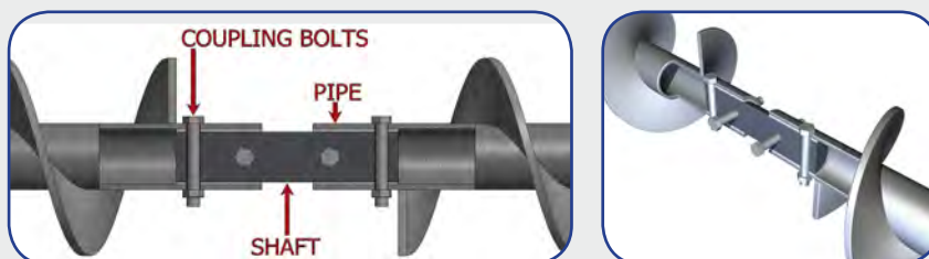
Standard Screw Construction (by Shaft Size)
