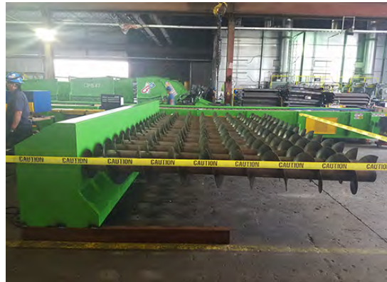
Screws are Installed at CP Manufacturing Facility and Ready for Testing
