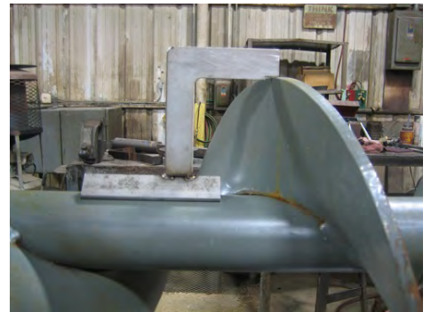
Special Gauge Verifies Correct OD of Screw
