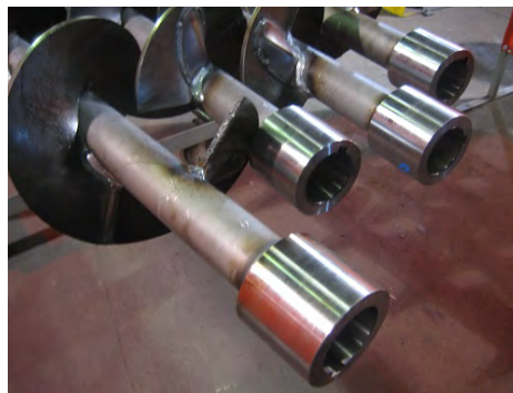
Drive End of Frac Blender Screws Utilize Special Keyed Hub
