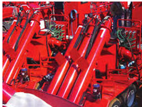
Multiple Screws Accurately Meter Sand to Blend Tank
