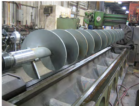
Screw is Checked in Lathe with Dial Indicators
