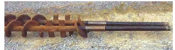
Existing Screws were Mounted on Smaller Center Diameter Pipe
