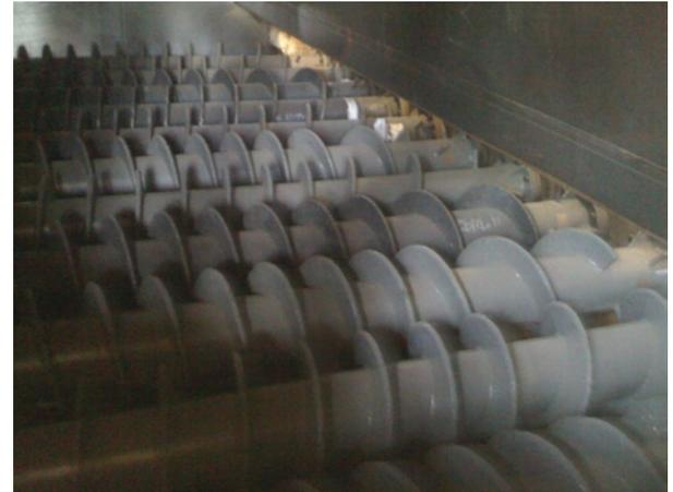
Live Bottom Bins consist of a storage hopper with multiple screws in the bottom. Hopper storage capacity is dependent on process requirements. The live bottom screws span the length and width of the storage hopper and are designed to remove the bulk materials at a consistent rate to feed the process. The Live Bottom Bins are designed to promote mass-flow and eliminate material bridging or arching in the hopper.
