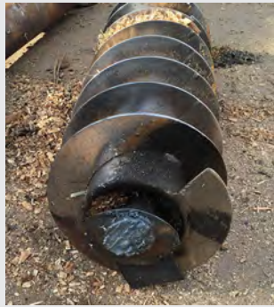
Old, Failed Screw with Weld-In Shafts That Had to Be Cut Off
