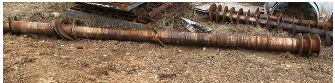
Old, Failed Screw with Flights Stripped Off
