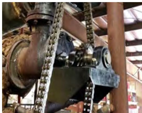
KWS Double-Pedestal Trough Ends Utilize Two Pillow Block Bearings
