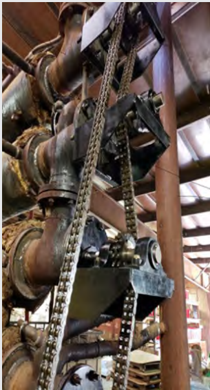
Steam-Jacketed Screw Conveyors are Stacked Vertically and Driven by a Common Drive Unit
