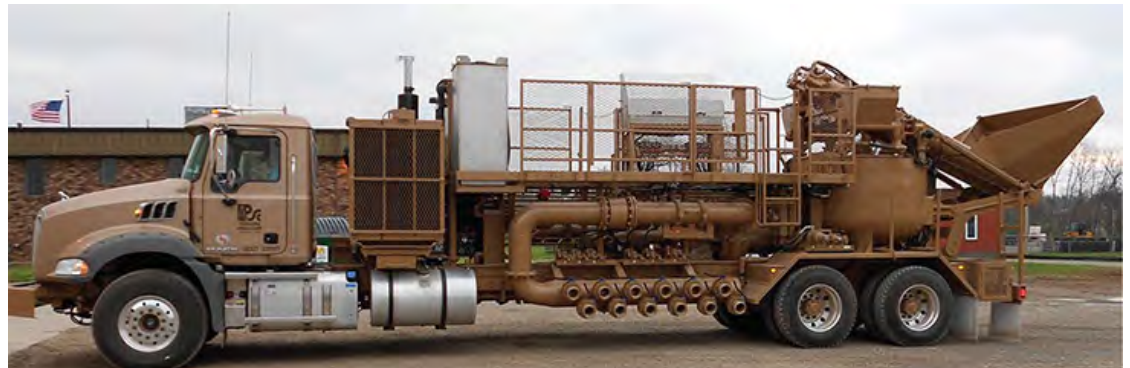
KWS Screws are Located inside the Tubular Housings on the Right Side of Blender Truck
