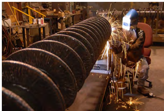
Welder Applies Weld-On Hardsurfacing Material to Flights
