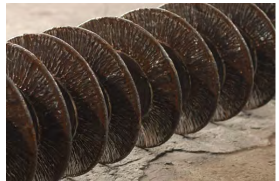
Hardsurfacing Reduces Abrasion on Flights
