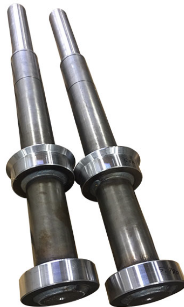
Shafts are Machined to Very Close Tolerances for Shrink Fit
