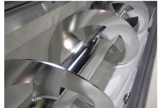
Screw Surfaces Electro-Polished to Mirror Finish with UHMW Trough Liner
