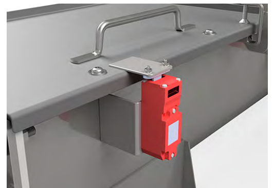
Machine Circuit is Enabled when Special-Shaped Actuator Key is Inserted in Switch
