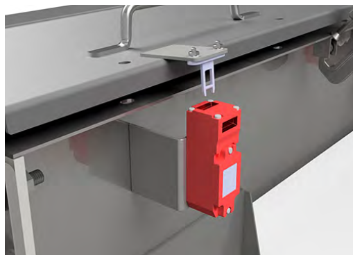
Machine Circuit is Broken when Special-Shaped Actuator Key is Removed from Switch
