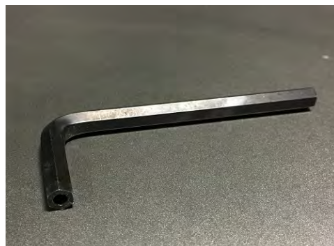
KWS Special Tool is Required to Properly Remove Covers
