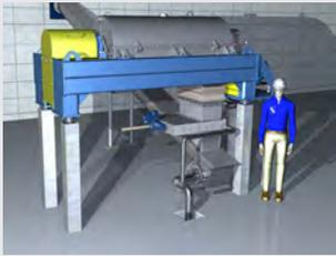
KWS Diverter Gate Located Under Centrifuge
