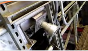
Milltronics XPP-5 Probe is Mounted to the Side of a Screw Conveyor
