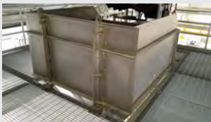
KWS Hopper with Load Stands Stores and Measures Bulk Materials
