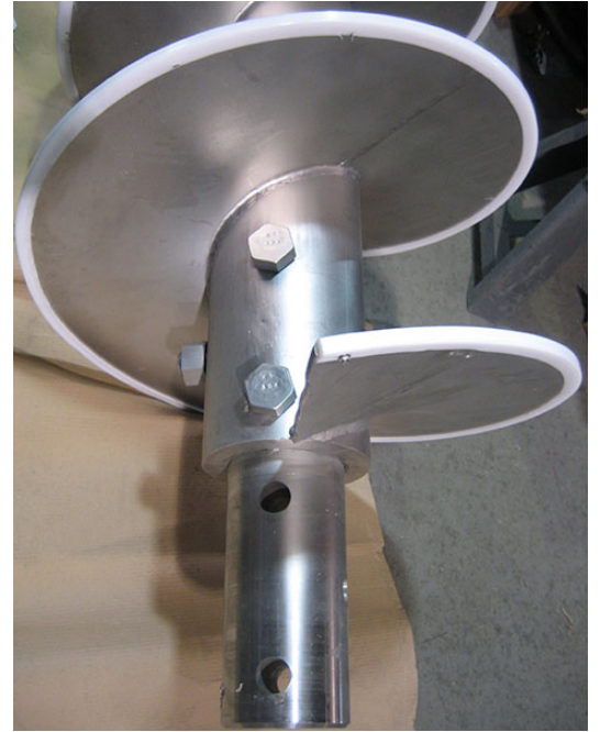
Flight Edging is Attached on Each End with a Single Bolt
