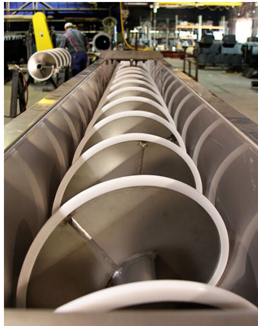
Flight Edging Provides Close-Clearance in Trough
