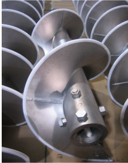
UHMW Flight Edging for Stainless Steel Screws
