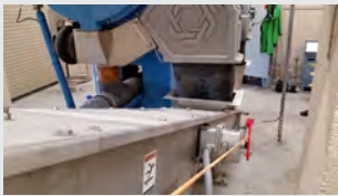
Control Unit Mounts to Side of Screw Conveyor
