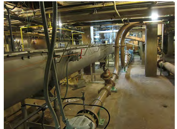
Single Control Unit Can be Used on Screw Conveyors up to 100-Feet in Length
