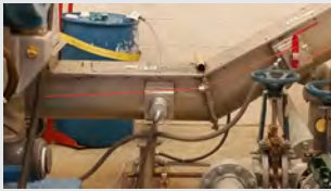
Cable Safety Stop Switch Control Unit can be Wired to Shut Off Multiple Conveyors
