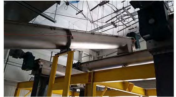
Multiple Screw Conveyors Utilizing Cable Safety Stop Switch Control Units
