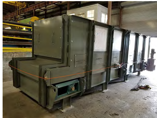
Safety Cable is Located on Three Sides of Belt Conveyor with One Control Unit
