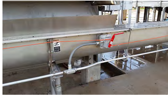
Guides are located Around the Conveyor to Support the Safety Cable
