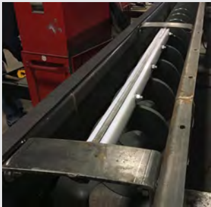
Hold Down Bolts to Sides of Trough for Easy Removal
