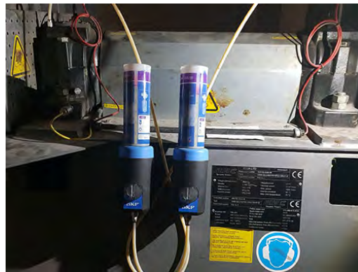
SKF System TLMR Can Be Used for Multiple Point Lubrication
