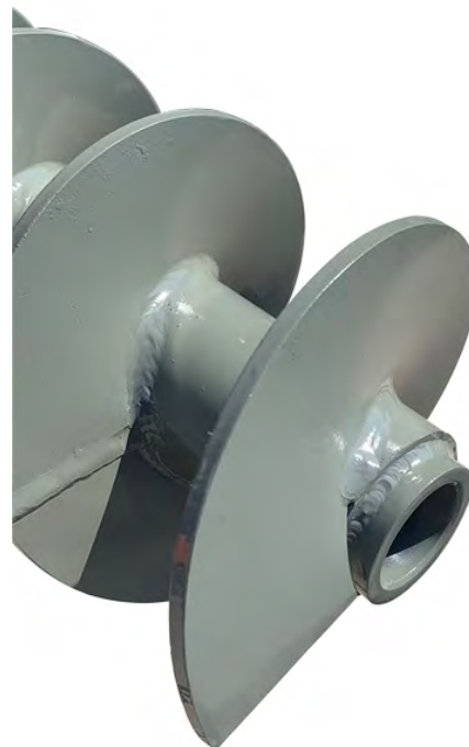
Bushing with Internal Spline is Welded in Place with Full Circumference Fillet Weld
