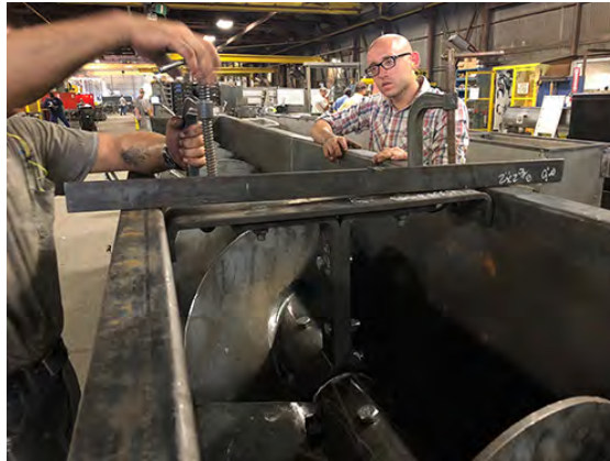
Step 8 – Hanger Being Raised in Trough Using C-Clamps
