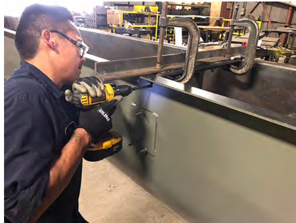
Step 10 – Hanger Holes on Each Side of Trough are Marked and Drilled
