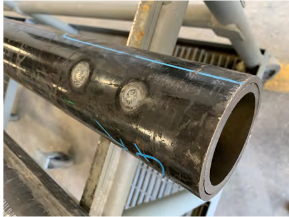
Proper Size and Location of Plug Welds
