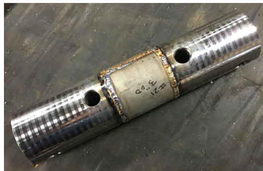
Coupling Shaft with Stellite Sleeve (Before Machining)
