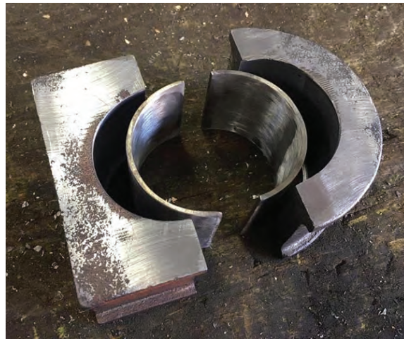
Style 216 Hanger Bearing with Stellite Sleeves (Before Welding)
