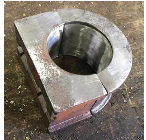
Style 216 Hanger Bearing with Stellite Sleeves (After Welding)
