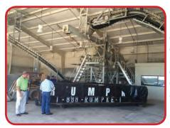
Before: Existing conveyor with only one discharge point overfilled one dumpster causing spillage and housekeeping issues.
