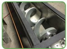
After: New high-strength KWS-350 shaftless spiral has a typical working life of over 10 years.
