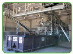
After: New KWS reversible screw conveyor has two discharge points for multiple dumpster loading and redundant operation.
