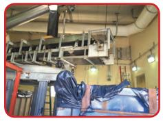
Before: Existing belt conveyor caused residual spillage and odors
