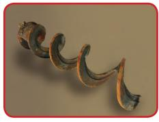
Before: Existing low strength carbon steel shaftless spiral weakened within 2 years and failed.
