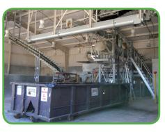
After: New KWS reversible screw conveyor has two discharge points for multiple dumpster loading and redundant operation.
