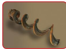
**Before:** Existing low strength carbon steel shaftless spiral weakened within 2 years and failed.
