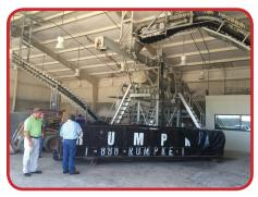
**Before:** Existing conveyor with only one discharge point overfilled one dumpster causing spillage and housekeeping issues.
